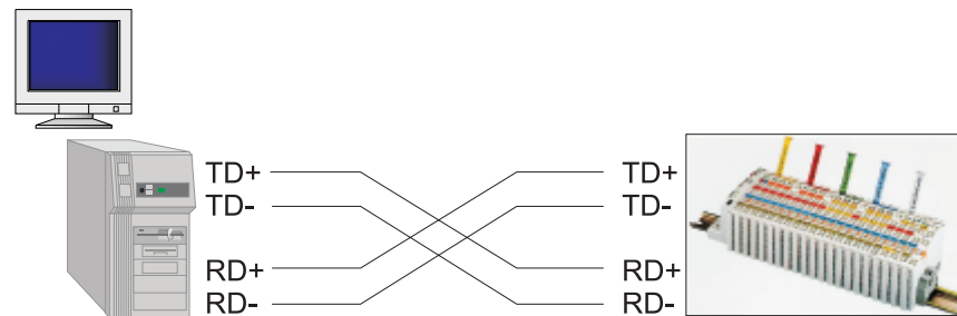
Fig. 5-2: Direct Connection of a Node with Crossover Cable
