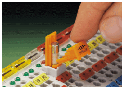
Fig. 2-16: Opening the fuse carrier
