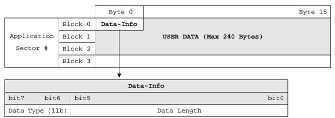
Data type is fixed with 11b which means "any other data" type of "Card Holder information" as MAD standard. And data length is including the data with ending zero "0", so the number of data byte sent by DF7XX reader is equal to data length with one less for RS232 output.
