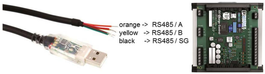
Figure 1: Connecting the RS385-USB converter to the EV CC Basic charge controller
